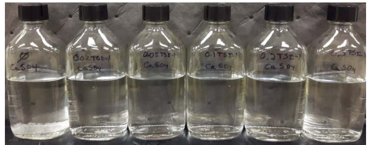
Figure 1. \text{CaSO}_4 decreases with increased concentration of TSI-1 (left to right: 0, 0.02, 0.05, 0.10, 0.20, 0.50 GPT).
